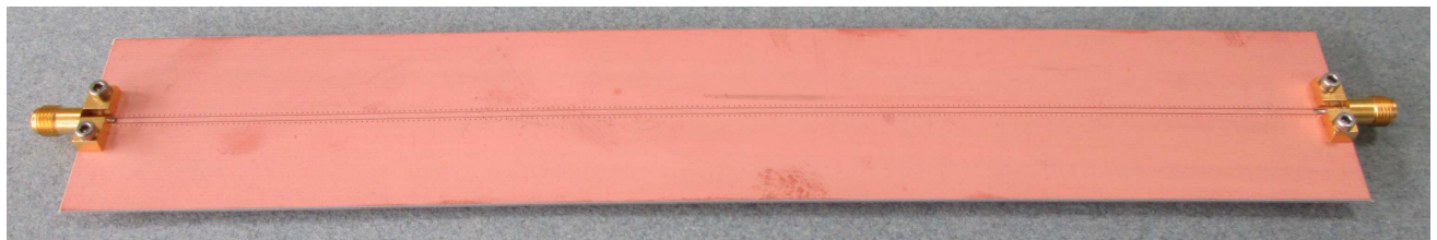
Figure 1 - 250mm long grouded CPW / 2.92mm connectors
