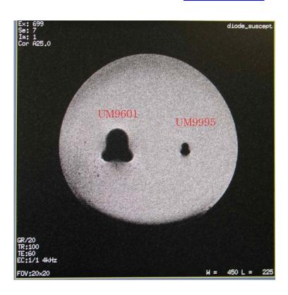
This is an actual Magnetic Image of the standard UM9601 and the specially constructed UM9995 PIN diode (in a 3T MRI system)
