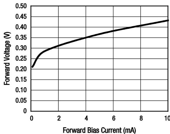
**Figure 2. Forward Voltage vs Forward Current**
