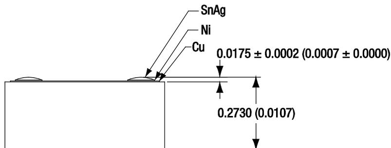
All measurements in millimeters (inches shown in parentheses).
