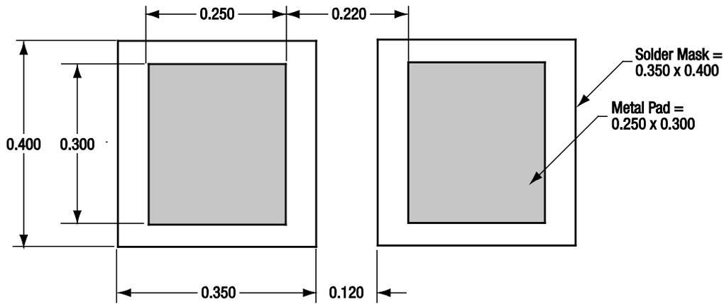
All measurements in millimeters
