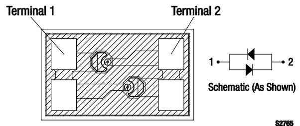
**Figure 1. SMS7621-092 Pinout (Bottom View)**
