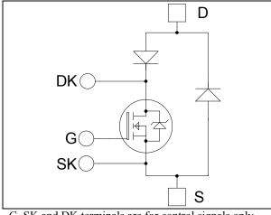
G, SK and DK terminals are for control signals only (not for power)
