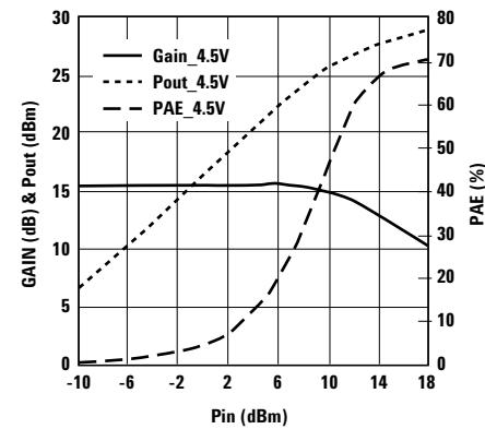
Figure 18. Small Signal Gain/Pout/PAE vs.
