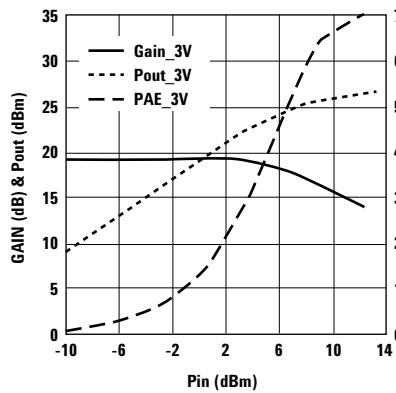
Figure 32. Small Signal Gain/Pout/PAE vs. Pin at Vds = 3V and Frequency = 900 MHz.
