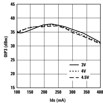
Figure 28. OIP3 vs Ids and Vds at 3.9 GHz.
