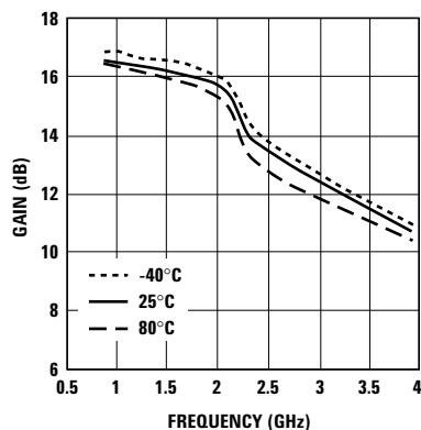
Figure 23. Gain vs. Temperature and Frequency at optimum OIP3.
