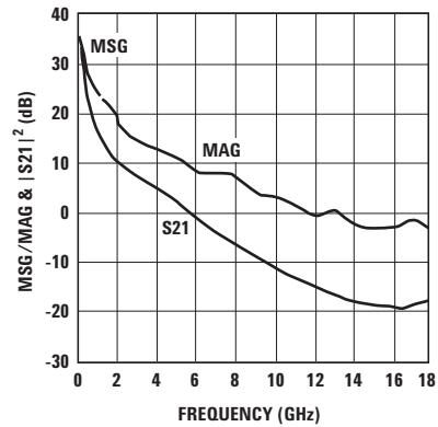
Figure 51. MSG/MAG & |S21|^2 vs. Frequency at 4.5V/200 mA.
