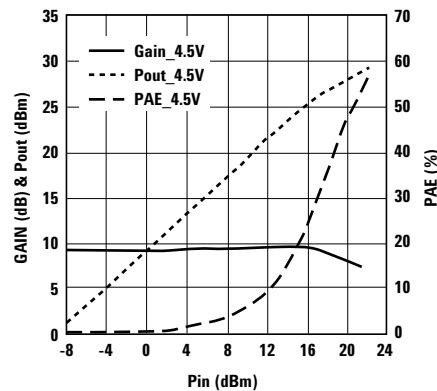
Figure 40. Small Signal Gain/Pout/PAE vs.
