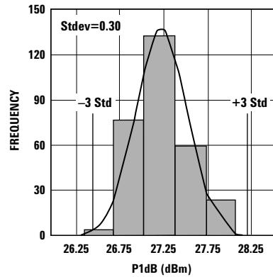
**Figure 3.** P1dB @ 2 GHz, 4.5V, 200 mA.
