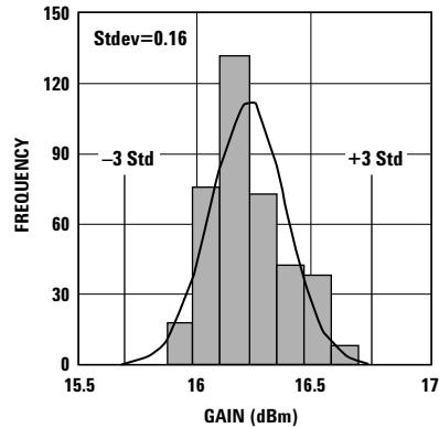
**Figure 4.** Gain @ 2 GHz, 4.5V, 200 mA.
