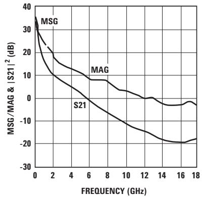
Figure 50. MSG/MAG &  $|S21|^2$  vs. Frequency at 4.5V/280 mA.
