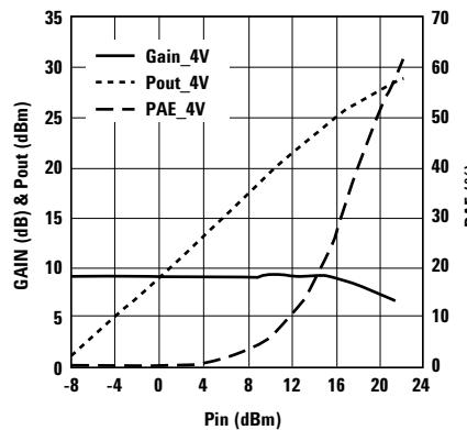
Figure 39. Small Signal Gain/Pout/PAE vs.
