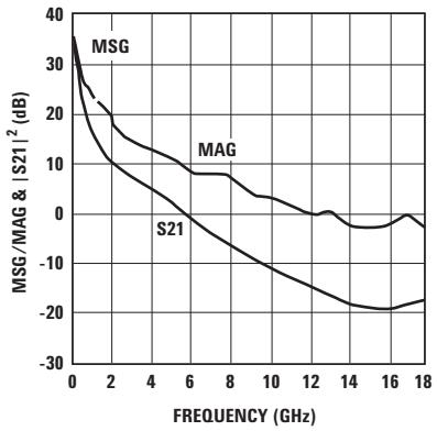
Figure 54. MSG/MAG &  $|S21|^2$  vs. Frequency at 3.0V/200 mA.
