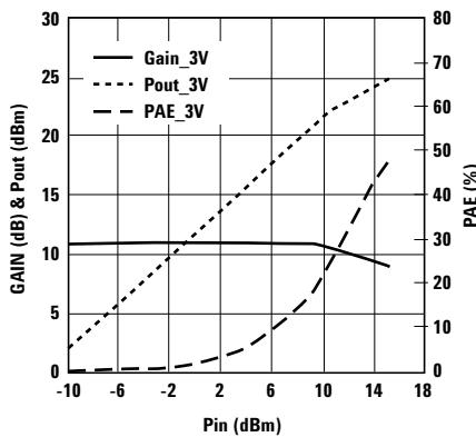
Figure 19. Small Signal Gain/Pout/PAE vs.
