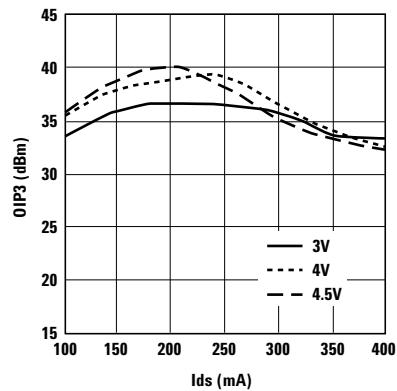
Figure 9. OIP3 vs. Ids and Vds at 3.9 GHz.
