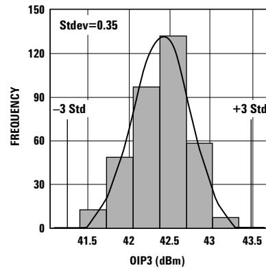
**Figure 2.** OIP3 @ 2 GHz, 4.5V/200 mA.
