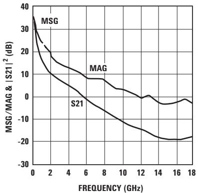
Figure 53. MSG/MAG &  $|S21|^2$  vs. Frequency at 4.0V/200 mA.
