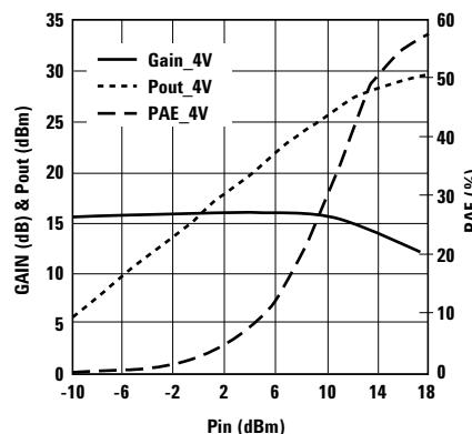
Figure 36. Small Signal Gain/Pout/PAE vs.
