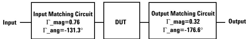
**Figure 1.** Block diagram of the 2 GHz production test board used for NF, Gain, OIP3 , P1dB, PAE and ACLR measurements. This circuit achieves a trade-off between optimal OIP3, P1dB and VSWR. Circuit losses have been de-embedded from actual measurements.
