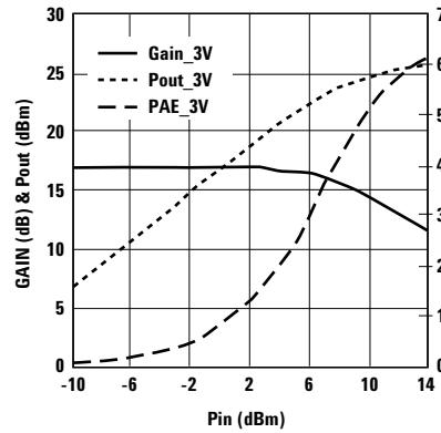
Figure 13. Small Signal Gain/Pout/PAE vs. Pin at Vds = 3V and Frequency = 900 MHz.
