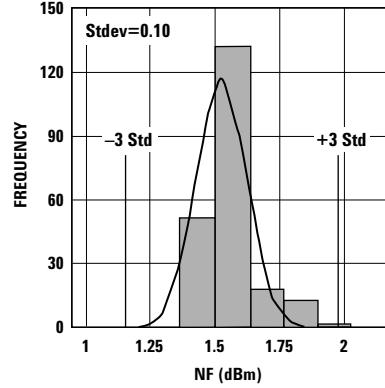
**Figure 5.** NF @ 2 GHz, 4.5V, 200 mA.
