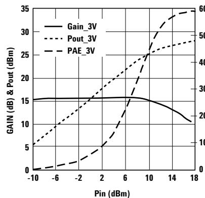
Figure 35. Small Signal Gain/Pout/PAE vs.
