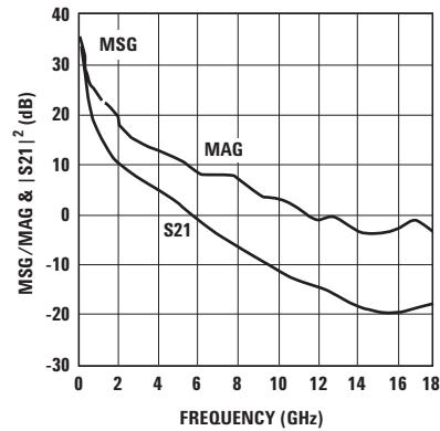
Figure 52. MSG/MAG & |S21|<sup>2</sup> vs. Frequency at 4.5V/120 mA.
