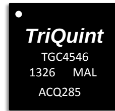
28-pin 5x5mm QFN package
