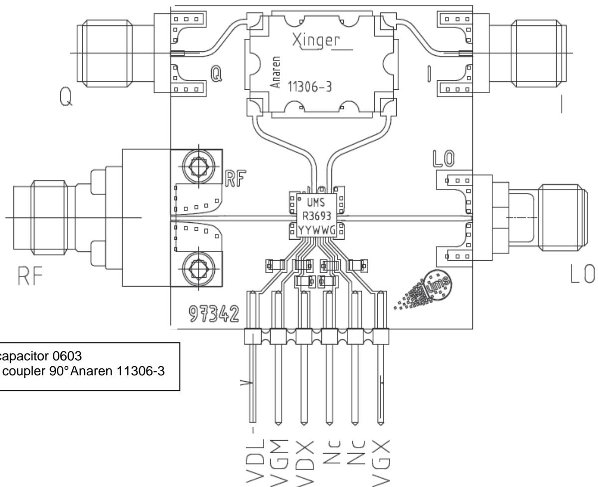
The DC connections do not include any decoupling capacitor in package, therefore it is mandatory to provide a good external DC decoupling on the PC board, as close as possible to the package.
