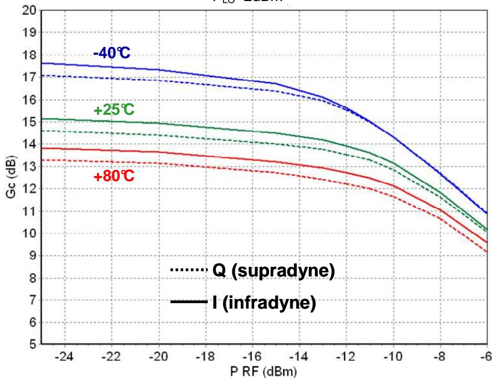
Compression vs  $P_{RF}$  (inf. & sup. Mode) @  $F_{RF}=26\text{GHz}$  &  $F_{IF}=2\text{GHz}$
