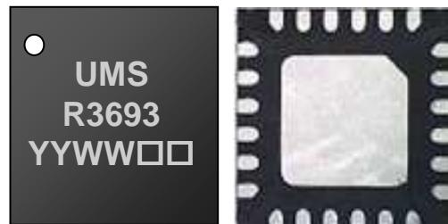
The circuit is manufactured with a pHEMT process, 0.25 $\mu$ m gate length, via holes through the substrate and air bridges.
