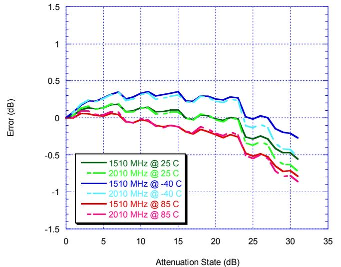
Note: Positive attenuation error indicates higher attenuation than target value
