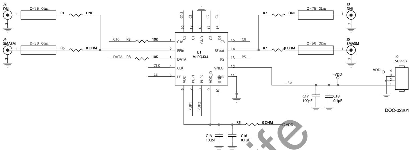
Note: Resistors on pins 1 and 3 are required and should be placed as close to the part as possible to avoid package resonance and meet error specifications over frequency
