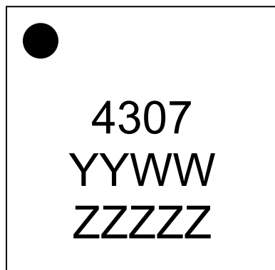
Figure 21. Top Marking Specifications
