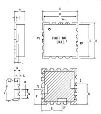
Pin Configuration1RF Output2Vcc3VtOthersGND
