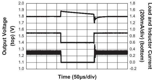
**Step-Down Converter Load Transient Response**
