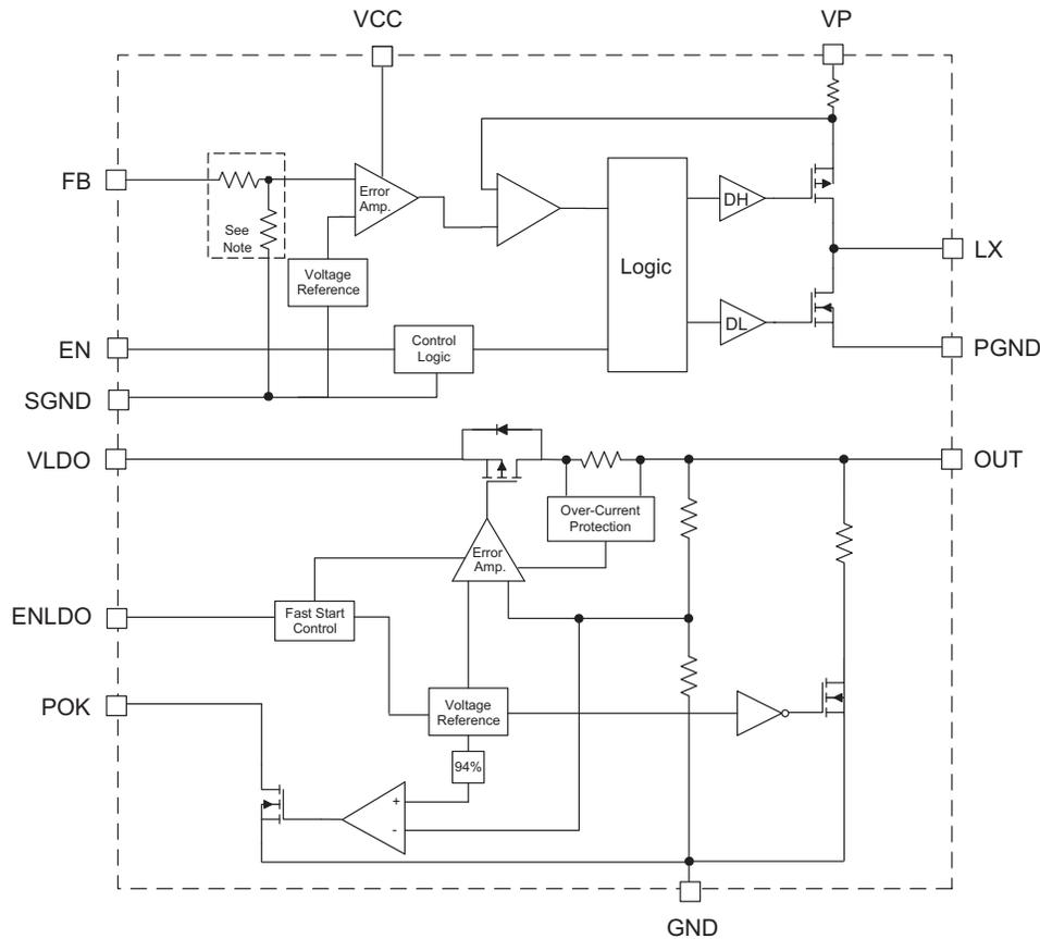
Note: Internal resistor divider included for □ 1.2V versions. For low voltage versions, the feedback pin is tied directly to the error amplifier input.
