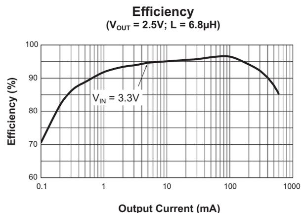
**Dual Channel, Step-Down Converter/Linear Regulator**
