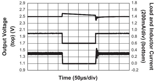
**Step-Down Converter Line Transient**
