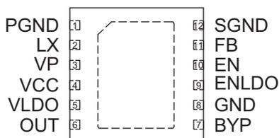
**AAT2506****1MHz Step-Down Converter/LDO Regulator****Absolute Maximum Ratings<sup>1</sup>**
