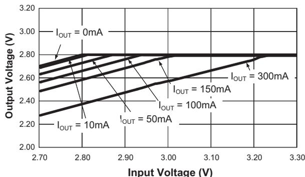
**LDO Dropout Voltage vs. Output Current**
