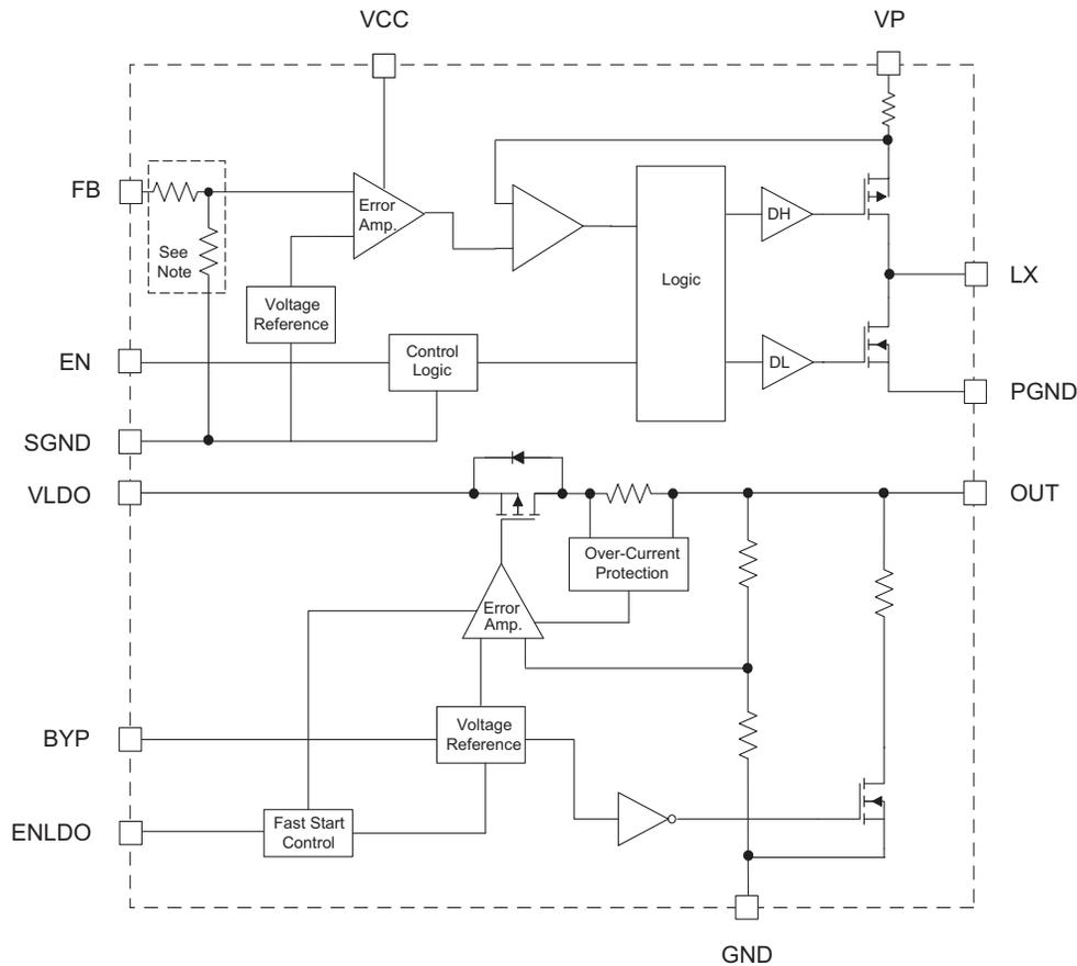
Note: Internal resistor divider included for  $\geq 1.2V$  versions. For low voltage versions, the feedback pin is tied directly to the error amplifier input.
