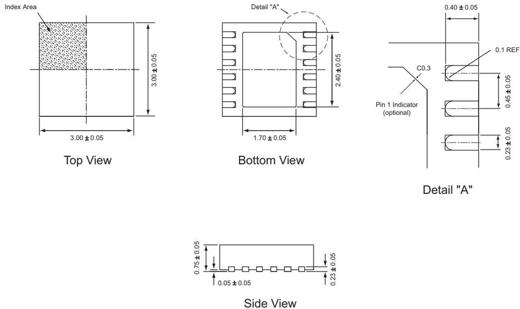
1. The leadless package family, which includes QFN, TQFN, DFN, TDFN and STDFN, has exposed copper (unplated) at the end of the lead terminals due to the manufacturing process. A solder fillet at the exposed copper edge cannot be guaranteed and is not required to ensure a proper bottom solder connection.
