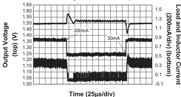
**Step-Down Converter Load Transient Response**
