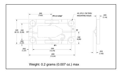
\*For the base model, only the IF1 port is connected. For the "-2" model, only the IF2 port is connected.
