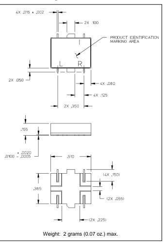
\* Dimensions are inches (millimeters) ±0.015 (0.38) unless otherwise specified.
