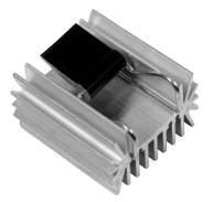
Ohmite's R2 Series (patent pending) heatsink provides a large surface area along with our C Series clipping mechanism to attach to a TO-220, TO-247, or TO-264 package. The self-aligning features of the clip assure secure attachment and enhanced thermal performance. Because no screws are required for device mounting, additional fins can be added to the rear side of the heatsink for increased total surface area in a more compact space.
