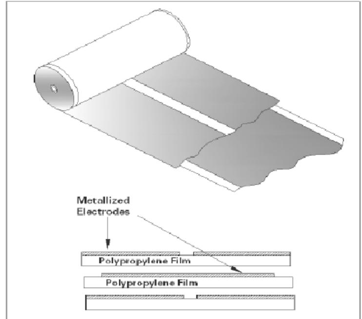
Regal-Beloit's GEM III capacitors are manufactured with high-grade metallized polypropylene film. This film is in the range of 5 to 10 microns thick, depending on the application, voltage, and conditions. The metallized electrode is several hundred angstroms thick.
