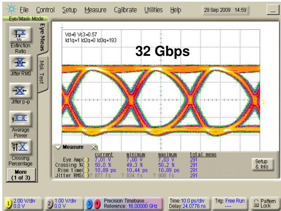
**Measured Data:**  $V_d = 7 \text{ V}$ ,  $V_{c1, 2, 3} = 0.7, 0.7, 0.8 \text{ V}$ ,
