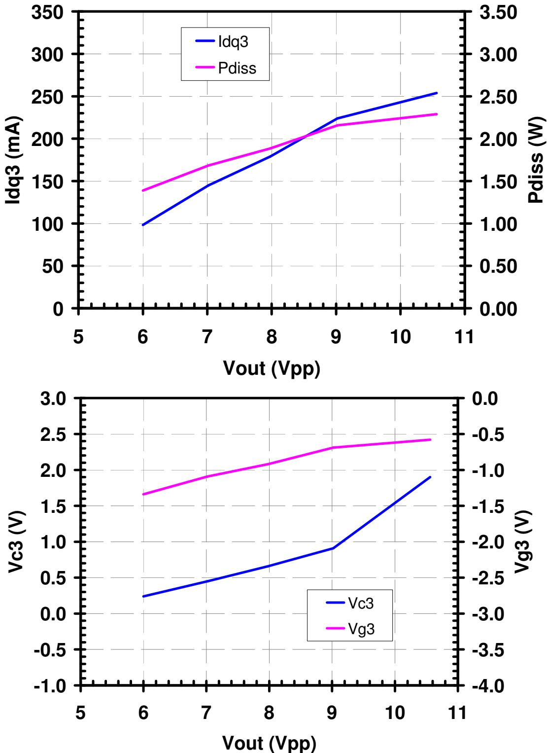
**Measured Data: Vin = 0.5 Vpp, 21.5 Gb/s, Vd = 7 V**
