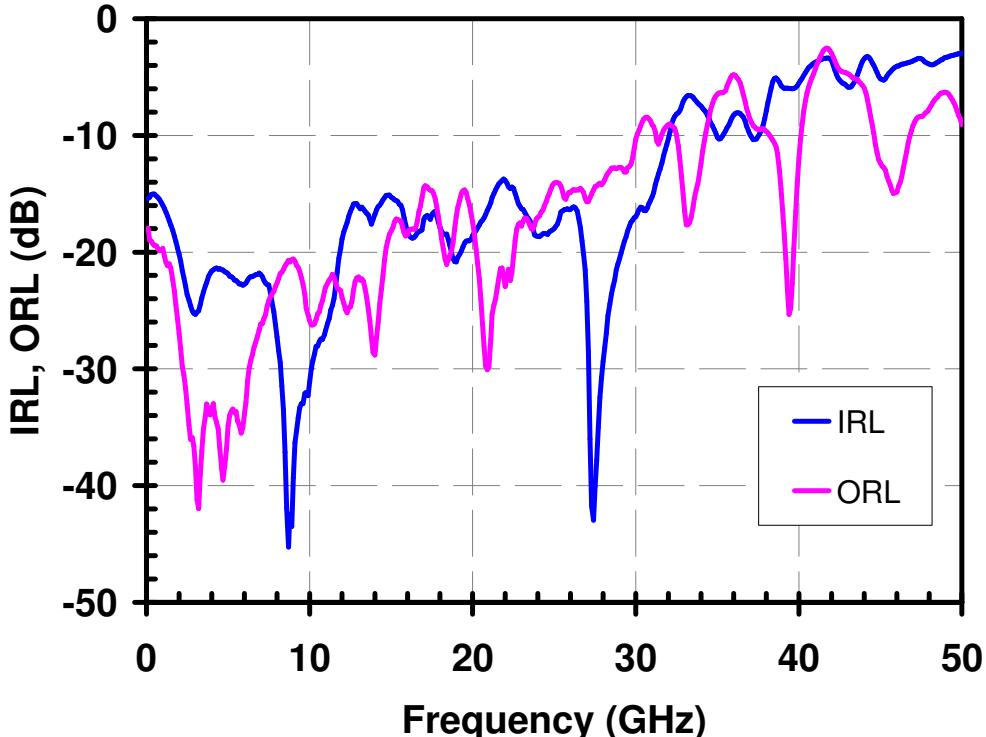
**Measured Data: Vin = 0.5 Vpp, 21.5 Gb/s, Vd = 7V**
