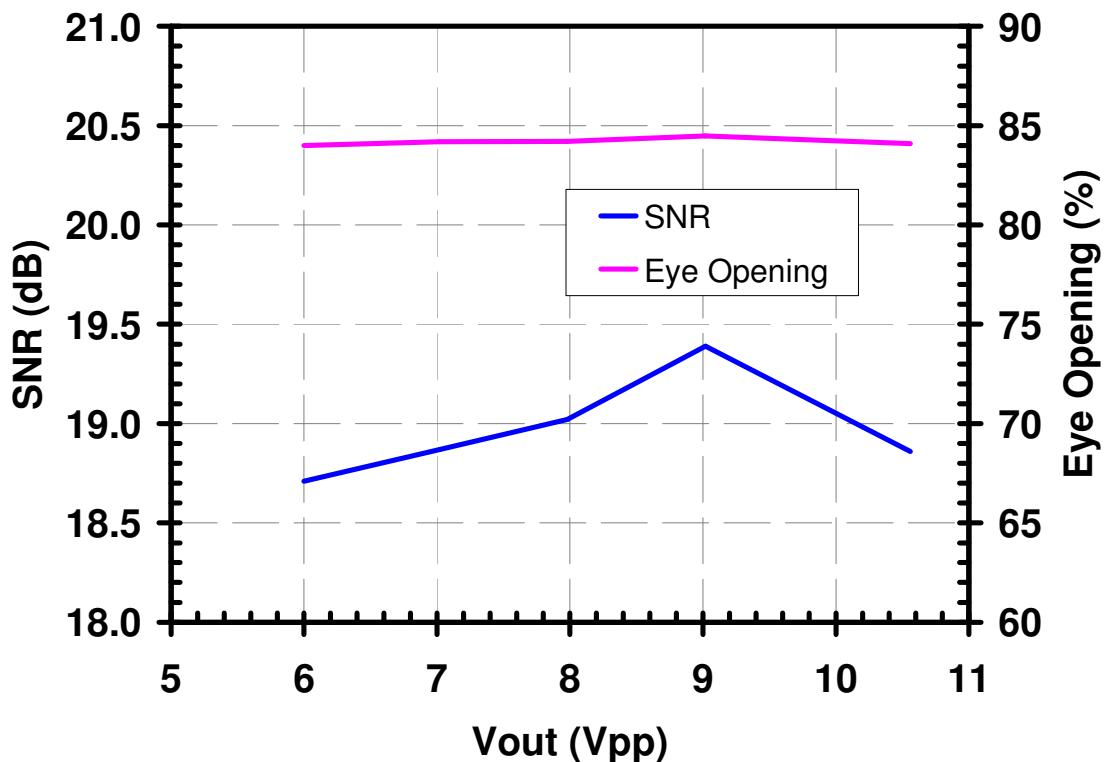
**Measured Data: Vin = 0.5 Vpp, 21.5 Gb/s, Vd = 7 V**
