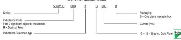
The above part number refers to a 506WLC Series 6.0 µH inductor, K tolerance (±10%, typ.), with Gold Plate (G), 200 mA, one piece in plastic box.
