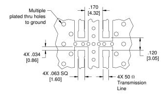
Dimensions are in Inches [Millimeters] 1P620S Rev A Mounting Footprint
