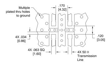
Dimensions are in Inches [Millimeters] JP520\* Mounting Footprint
