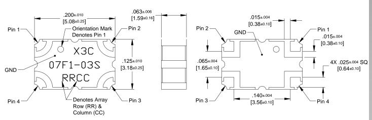
Dimensions are in Inches [Millimeters] X3C07F1-03S Mechanical Outline
