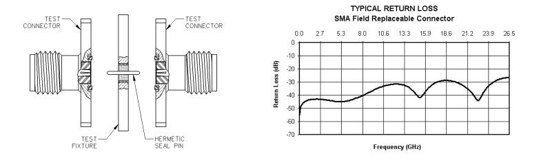
Although Johnson Components<sup>™</sup> does not publish a VSWR specification for field replaceable connectors, typical connector VSWR can be expected to be less than 1.1 + .01f (f in GHz). A VSWR specification is not stated because an industry standard method for testing field replaceable connectors does not exist. The actual performance of the connector is dependent upon the application for the following reasons:
