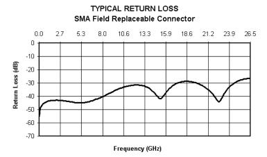
Although Johnson Components<sup>™</sup> does not publish a VSWR specification for field replaceable connectors, typical connector VSWR can be expected to be less than 1.1 + .01f (f in GHz). A VSWR specification is not stated because an industry standard method for testing field replaceable connectors does not exist. The actual performance of the connector is dependent upon the application for the following reasons:
