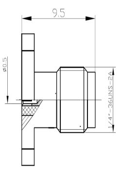
Electrical Specification: Impedance: 50 ohms Frequency: DC-18GHz Temperature Range: -65-+165Deg.C Durability: 500 cycles min. All materials are RoHS compliant.
