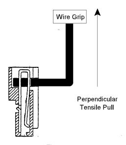
Figure 6 Termination Tensile Strength
