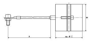
2. Parallel (aligned to corrugated copper tube cable) grounding cable connection
