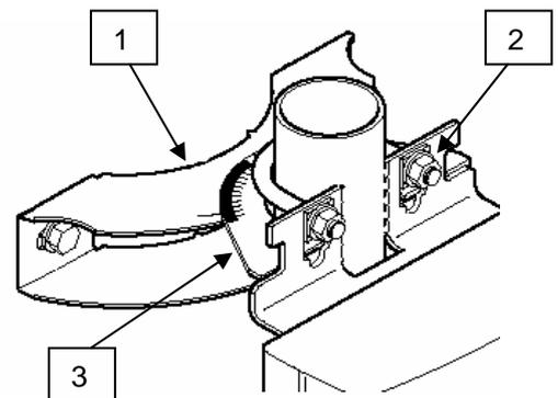
Mount the sidetilt bracket **1** to the wall.
