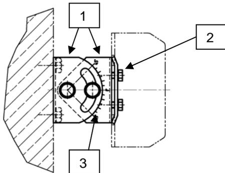
Attach pre-assembled sidetilt bracket **1** to the antenna with bolts and star washers **2**.
