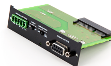
Industrial Serial Expansion Card (#CG1102-11920)
