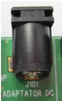
Figure 6. Main Supply Adapter
