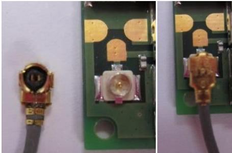
Figure 24. UFL Connector for use with a GSM/WCDMA Antenna
