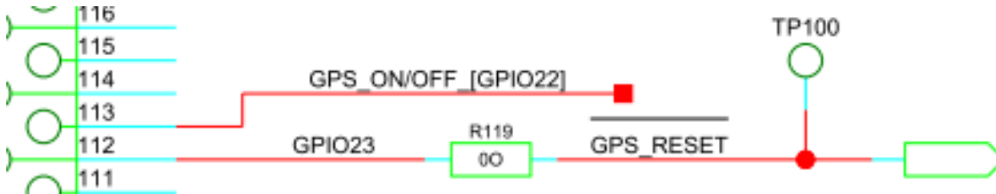
Figure 22. TP100 RESET Test-Point schematic
