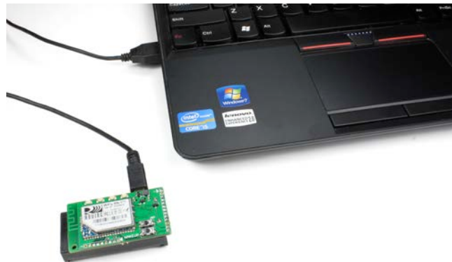
RN-171-EK Evaluation Board Hardware Setup
