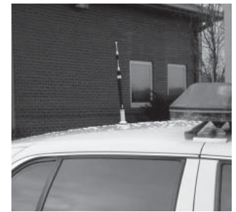
The MEFC24005 (top and left) elevated feed antenna is ideal for public safety vehicles with overhead light bars that often obstruct the RF signal.
