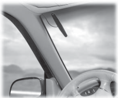
APDM5920U, vertical installation. The antenna can also be installed horizontally.
