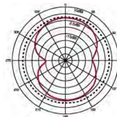
Elevation Plane (cut perpendicular to the antenna and parallel to the polarization)
