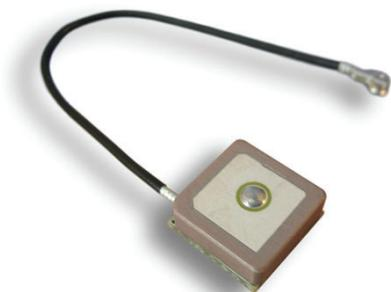
The Compact 1357D Embedded GPS antenna is ideal for GPS enabled ruggedized PDAs, laptops and portable GPS Handhelds. The 1357D antenna features a compact ceramic patch element, ESD circuit protection, a low noise amplifier and a SAW filter, enabling the 1357D to provide great out-of-band signal rejection performance, consistent and clear signal while minimizing loss-of-lock in an extremely small form factor.
