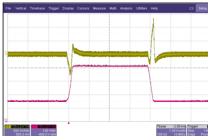
Figure 6: Output voltage response to step-change in input voltage (180V - 425V - 180V), at 6.25A load current. Load cap: 15µF tantalum capacitor and 1uF ceramic cap. Ch 1: V_{out} (1V/div), Ch 2: V_{in} (100V/div).
