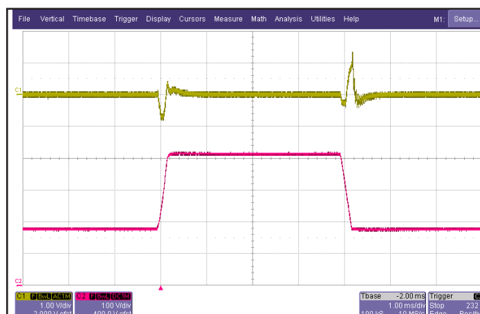
Figure 6: Output voltage response to step-change in input voltage (180V - 425V - 180V), at 6.25A load current. Load cap: 15μF tantalum capacitor and 1μF ceramic cap. Ch 1: V out (1V/div), Ch 2: V in (100V/div).
