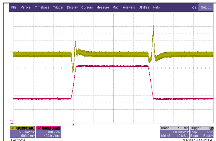
Figure 6: Output voltage response to step-change in input voltage (180V - 425V - 180V), at 10.7A load current. Load cap: 15μF tantalum capacitor and 1μF ceramic cap. Ch 1: V out (500mV/div), Ch 2: V in (100V/div).
