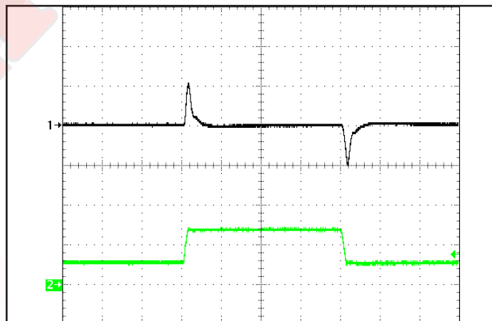
Figure 12: Output voltage response to step-change in input voltage (500V/ms), at full load current. Load cap: 100 \mu F electrolytic output capacitance. Ch 1: V_{out} (5V/div), Ch 2: V_{in} (50V/div).
