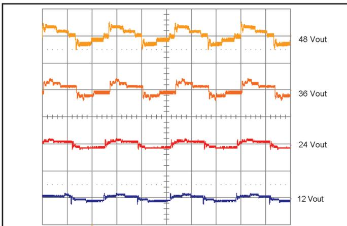
Figure 11: Output voltage response for 12V, 24V, 36V, and 48Vout to step-change in load current (50-75-50% of Iout max;  $di/dt=0.1A/\mu s$ ). Load cap: 100 $\mu$ F, 100m $\Omega$  ESR tant, Vout (2V/div).
