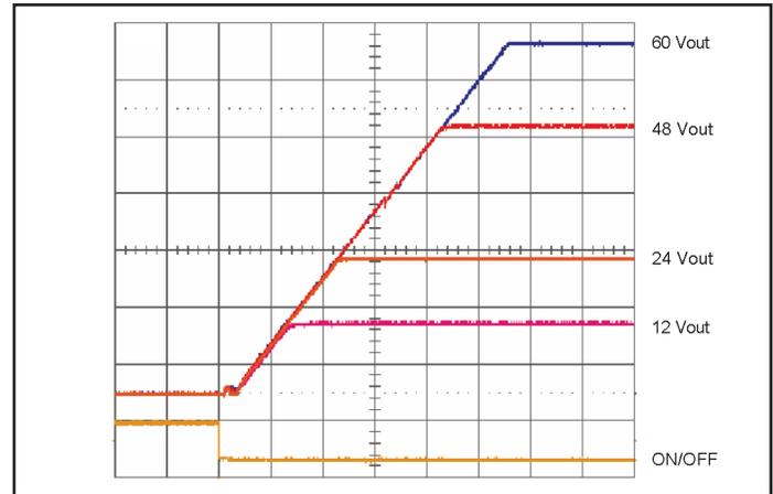
Figure 8: Turn-on transient at full load (20ms/div).
