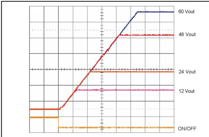
Figure 7: Turn-on transient at zero load (20ms/div).
