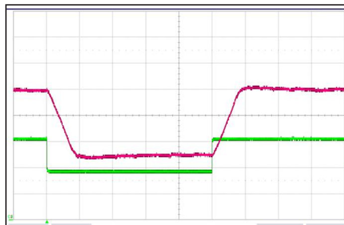
Figure 12: Output Current vs Iset pin voltage dynamics; 28Vin 10Vout (5mS/div). Top Trace: Output Current (2A/div). Bottom Trace: Iset pin voltage (200mV/div).
