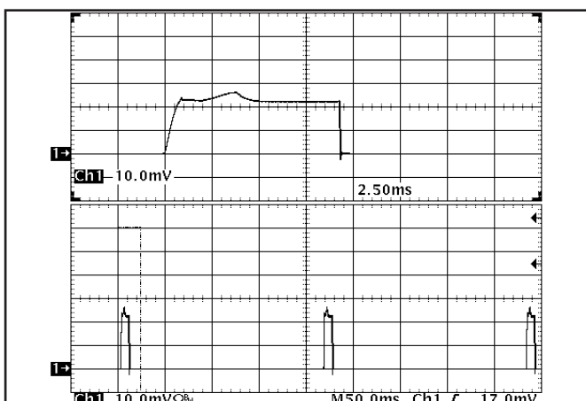
Figure 18: Load current (50A/div) as a function of time when the converter attempts to turn on into a 1\ \text{m}\Omega short circuit. Top trace (2.5ms/div) is an expansion of the on-time portion of the bottom trace.
