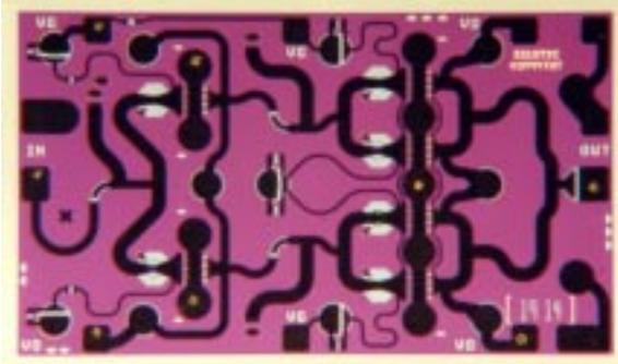
The TriQuint TGA1073C-SCC is a two stage PA MMIC design using TriQuint's proven 0.25  $\mu$ m Power pHEMT process to support a variety of millimeter wave applications including point-to-point digital radio and point-to-multipoint systems.
