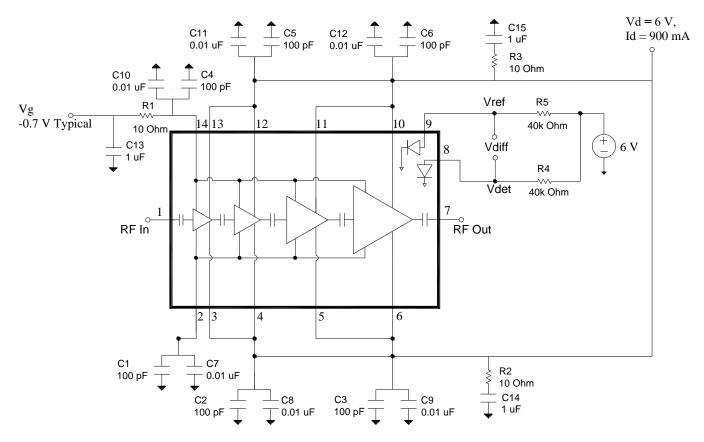
Vd must be biased from both sides. Vg can be biased from either side.
