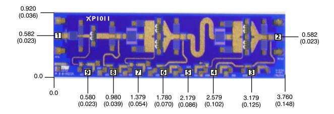
Units: millimeters (inches) Bond pad dimensions are shown to center of bond pad. Thickness: 0.110 +/- 0.010 (0.0043 +/- 0.0004), Backside is ground, Bond Pad/Backside Metallization: Gold All Bond Pads are  $0.100 \times 0.100 (0.004 \times 0.004)$ .
