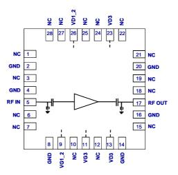
UMS develops a very high power packaged monolithic 7-16GHz power amplifier featuring up to 29dBm output power at  $P_{-1dB}$  gain compression. The high 20dB gain associated with the high linearity of 37dBm make of this circuit a very versatile part for high performance systems. Moreover it is proposed in standard surface mount package and integrates ESD protection. The overall power supply is of 5.0V/700mA.
