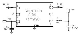
Important: Sequencing bias circuit required to Vgg and Vddl Vdd=+11V, Idd=400 mA. Adjust Vgg and Vdd slightly for best IP3. The resistance between Vgg and Pin 3 should be less than 200 lbm
