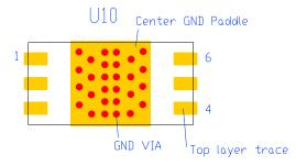
Note: GND vias are metallic plated and connected to ground layer on back side
