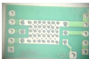
Fig. 2 Dispensed solder paste
