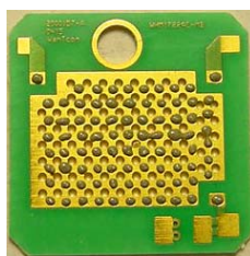
Fig. 2 Dispensed solder paste
