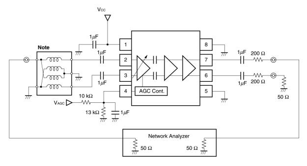
Note Balun Transformer: TOKO 617DB-1010 B4F (Double balanced type)
