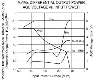
Conditions  $f_1 = 44 \text{ MHz}$   $f_2 = 45 \text{ MHz}$   $Z_L = 250 \Omega$   $V_{out} = 2.0 \text{ V}_{P\text{-P}}/\text{tone Constant}$  measurement circuit 4
