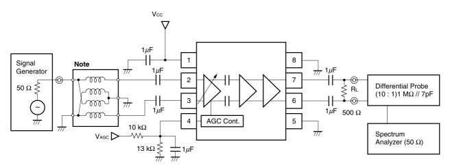
Note Balun Transformer: TOKO 617DB-1010 B4F (Double balanced type)
