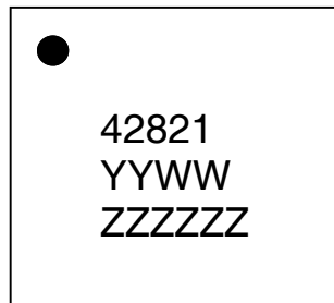
Figure 17. Top Marking Specification
