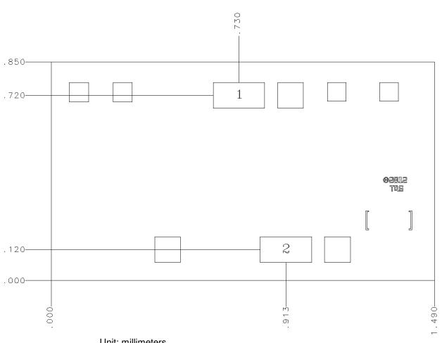
Unit: millimeters Thickness: 0.085 Die x, y size tolerance: +/- 0.050 Chip edge to bond pad dimensions are shown to center of pad Ground is backside of die
