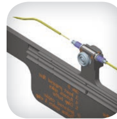
Insert Second Fiber and Actuate Crimp
